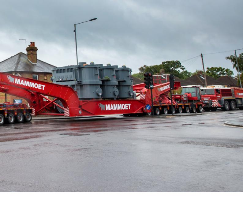
Girder frame trailers easily overcome height and weight restrictions on route, such as low or weak bridges, weight-sensitive surfaces, and overhead cables. Holding loads lower to the ground during transportation allows them to pass under lower bridges and spread weight for more even weight distribution on structures. Subsequently more - and potentially shorter - routes are available.
