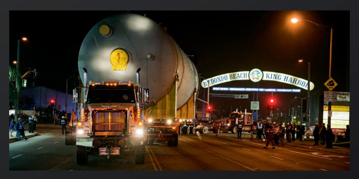
named California Dollies. These dollies got their name because they were built with specific axle spacing, compliant with Californian regulations. Once the coke drums were loaded on to the dollies, the SPMTs were transported back to the port to collect the second set a week later.
