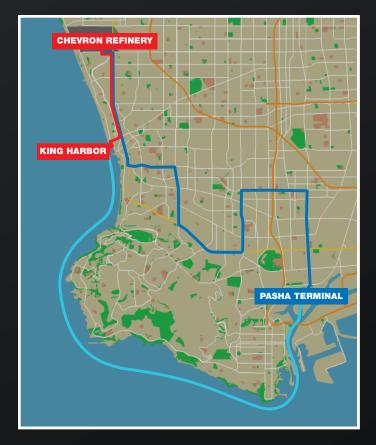
The coke drums were transported 26 nautical miles, by barge, from Pasha Terminal to King Harbor. From there they were taken, in pairs, by road over the last 4.5 miles to the refinery. The alternative route was 18 miles by road. The Mammoet approach saved three weeks transportation time and reduced the disruption to residents along the alternative route.
