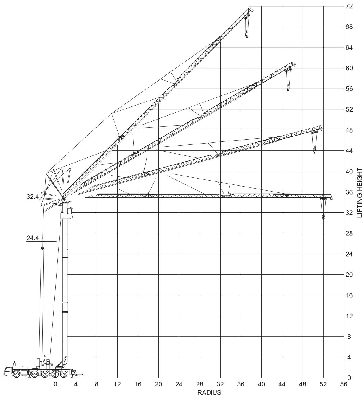
Crane dimensions are in millimeters. Radius diagram dimensions are in meters.
