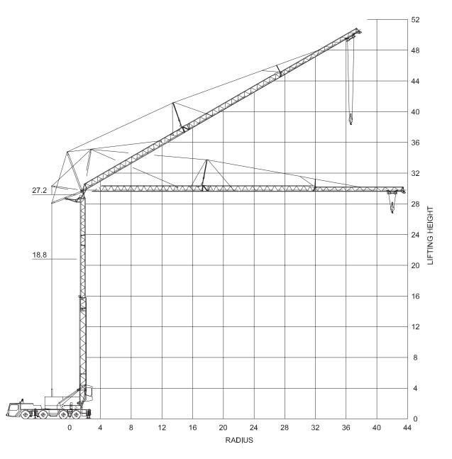
Crane dimensions are in millimeters. Radius diagram dimensions are in meters. The content in this document is mentioned for reference use only. Values may differ from current data. Always contact Mammoet for current project calculations.
