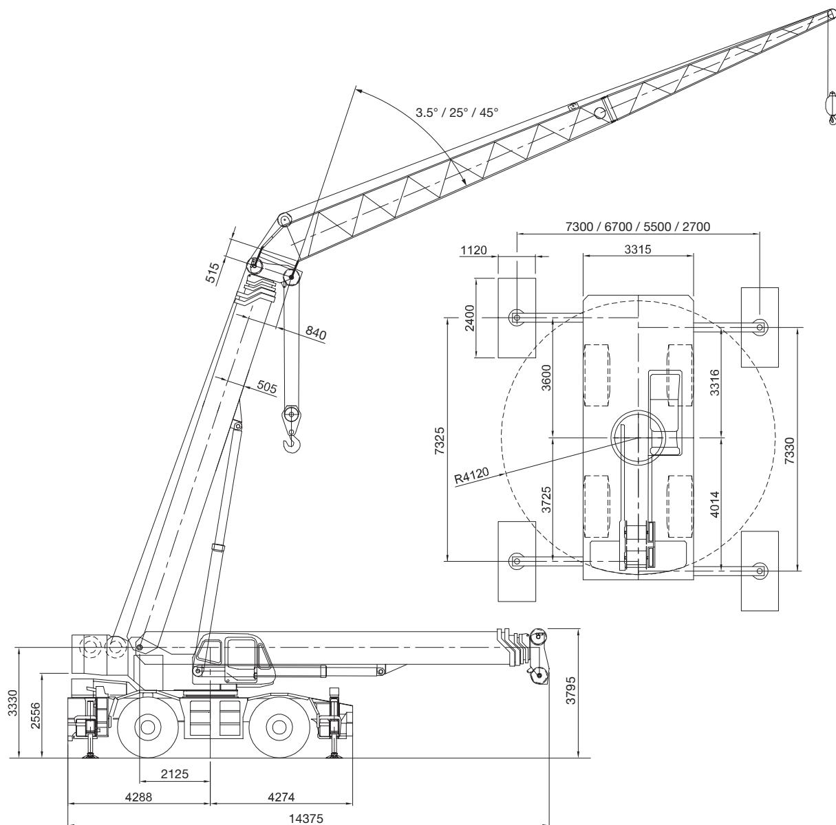
Dimensions are in millimeters.
