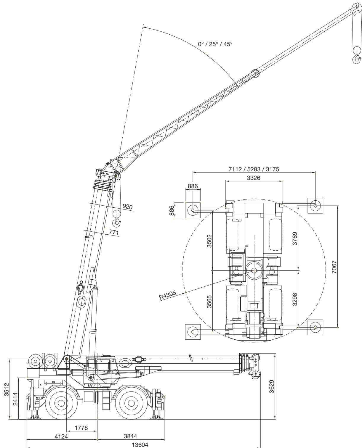
Dimensions are in millimeters.
