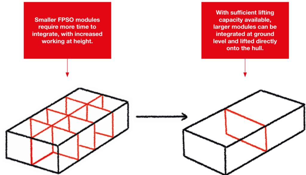
Connecting two modules rather than eight means a 400% decrease in surface area that must be joined together, and therefore huge savings on integration time and working at height. However, lifting technology must be found that can install these heavier modules.
