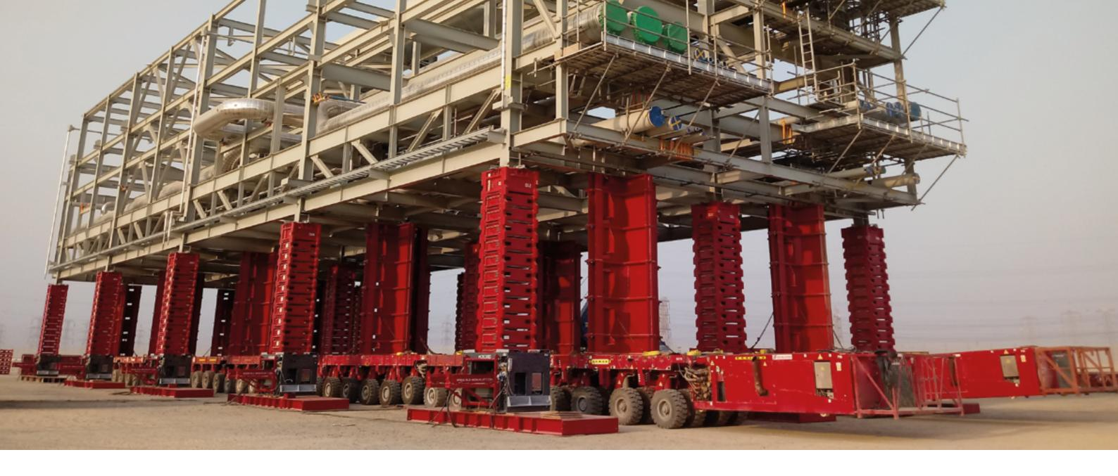
The Mega Jack 300 offers a quick, flexible solution for projects where time and space is limited. Jacking operations can be completed in as little as one hour, and the system can easily be moved or reconfigured on site.
