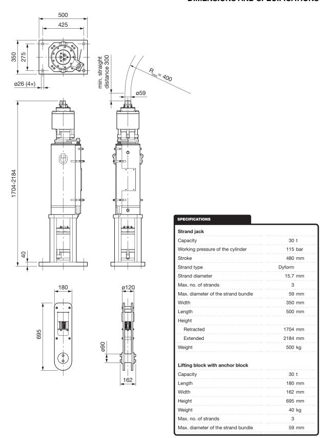
$\label{eq:definition} Dimensions are in millimeters, t = metric tons.$  The content in this document is mentioned for reference use only. Values may differ from current data. Always contact Mammoet for current project calculations.
