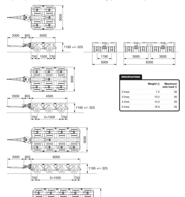
Dimensions are in millimeters.
