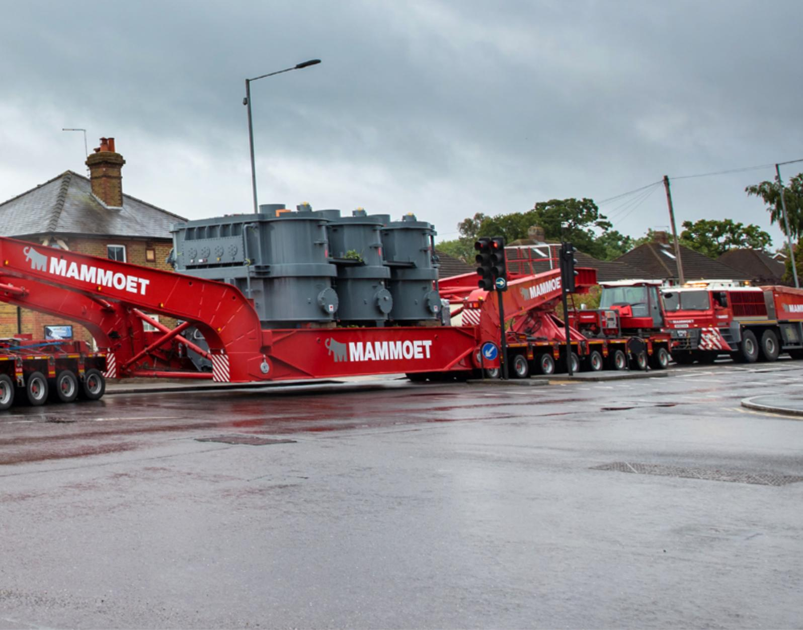
Girder frame trailers easily overcome height and weight restrictions on route, such as low or weak bridges, weight-sensitive surfaces, and overhead cables. Holding loads lower to the ground during transportation allows them to pass under lower bridges and spread weight for more even weight distribution on structures. Subsequently more - and potentially shorter - routes are available.
