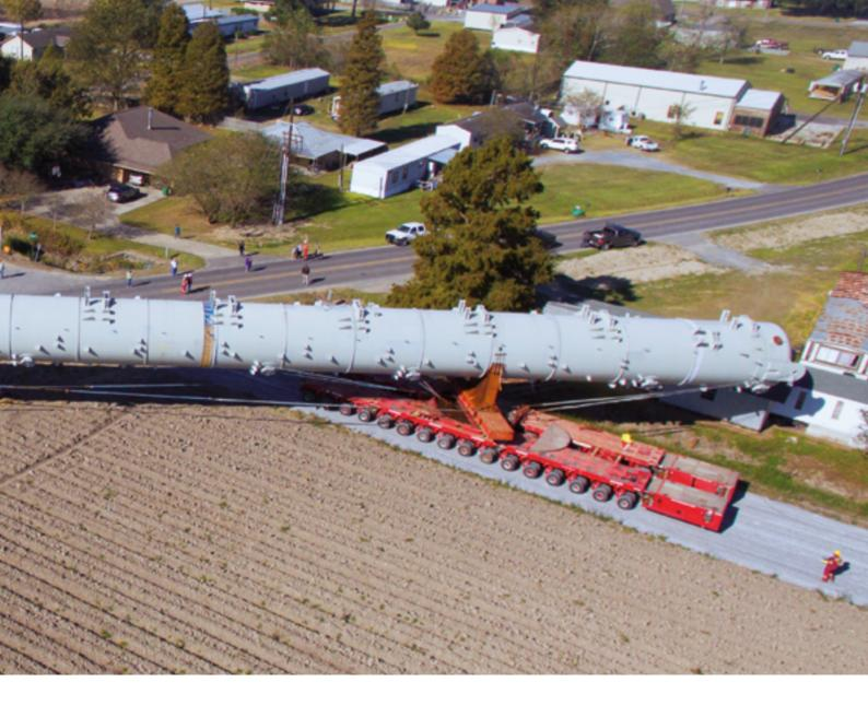
This means Mammoet's SPMTs can be mobilized swiftly around the world, meeting capacity demands from the smallest to the largest projects. Our fleet offers a variety of configurations, allowing customers to choose the right configuration for each job, based on 4, 5, 6 and 8 axle line trailer units. We can also offer SPMTs with an adjustable widening system as well as SPMTs adapted to extreme hot and cold temperatures.
