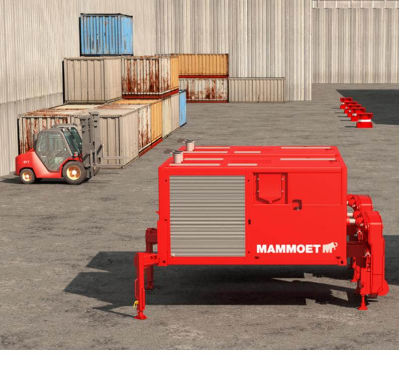
With industries around the world increasingly relying on heavy transport to facilitate construction projects at ever-larger scales, Mammoet Trailer Power Assist saves time, saves fuel and reduces the equipment requirement for heavy transport operations.
