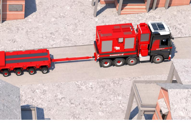
Mammoet Trailer Power Assist's Power Pack Unit uses a 1,000 horsepower diesel engine that is compliant with the latest emission control regulations.
