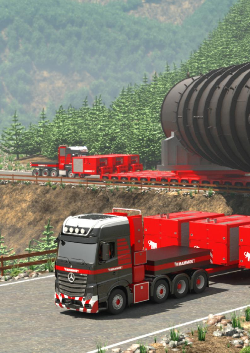
Mammoet's new Trailer Power Assist system brings deadlines forward, improving efficiency and safety while significantly lowering the carbon footprint in engineered heavy transport.
