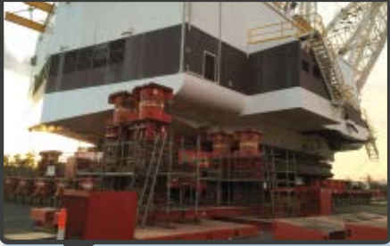
PHOTO 1 JACKING UP OF DRAGLINE ONTO SPMT
